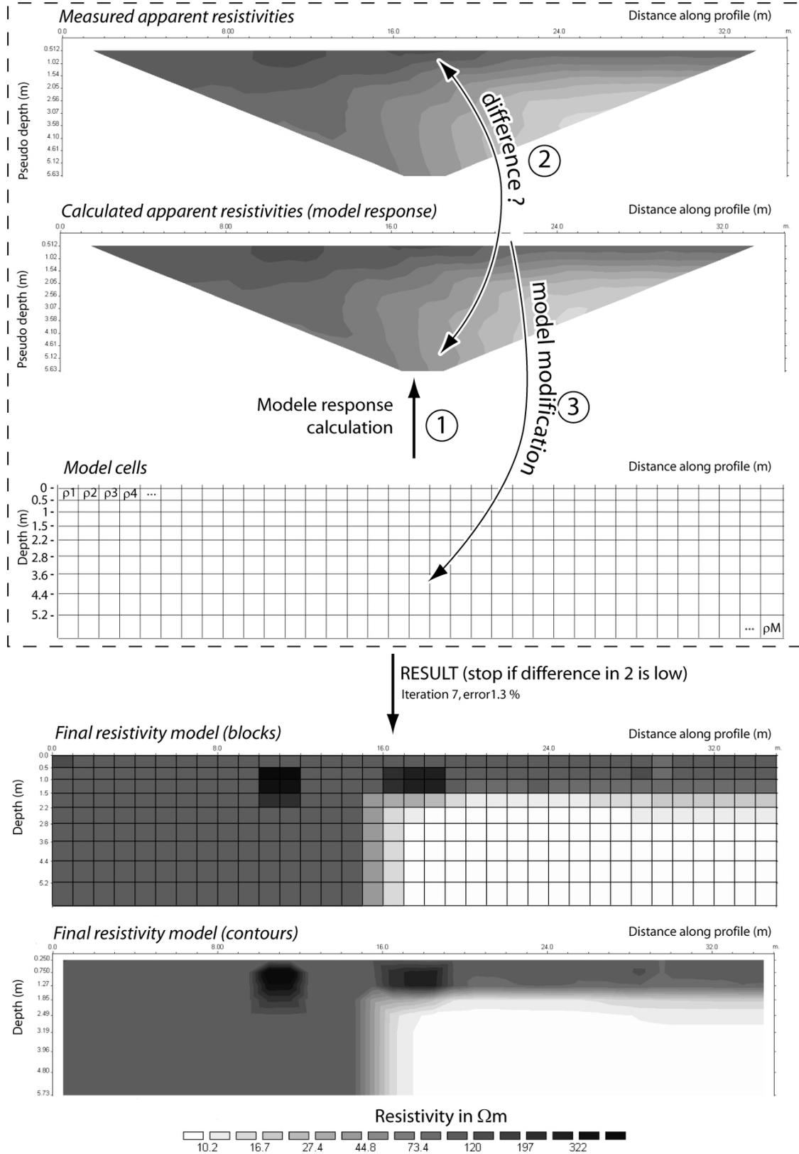
Figure 8: Principle of resistivity inversion (modified from Marescot, 2006)
