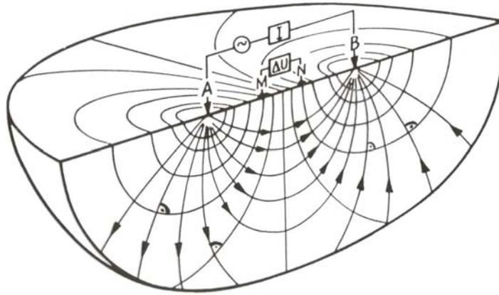
Figure 2: Equipotential surfaces and associated current lines for two current electrodes
