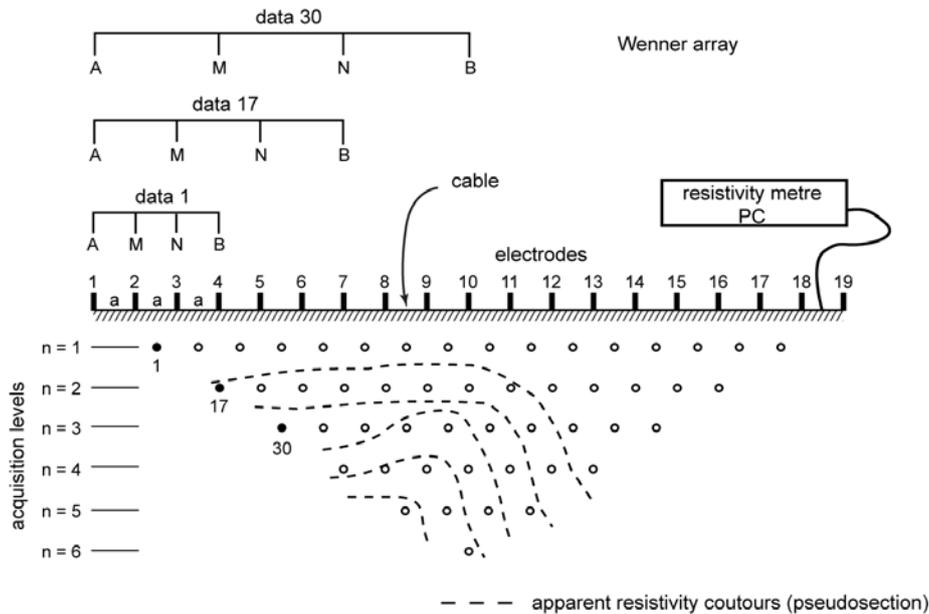
Figure 5: Principle of 2D electrical resistivity tomography and pseudosection (modified from Marescot, 2006)
