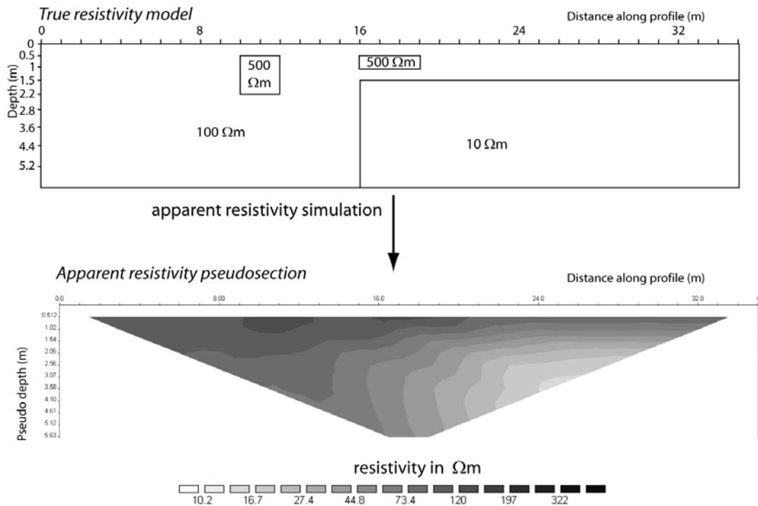
Figure 6: Example pseudosection for a simple resistivity model (modified from Marescot, 2006)
