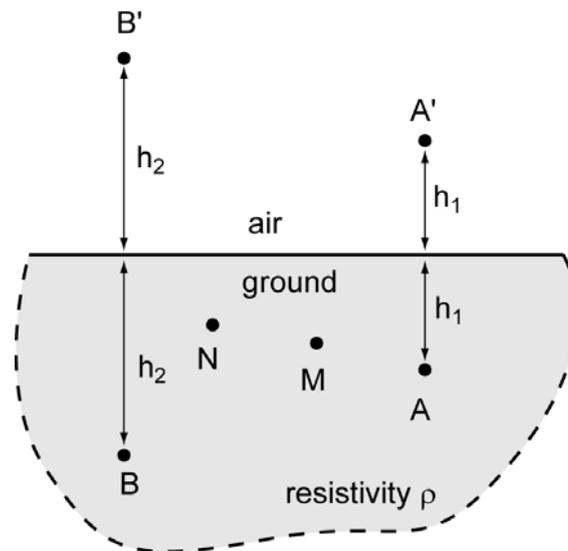
Figure 4: Electrode array frequently used in surface electrical prospecting (modified from Marescot, 2006)
