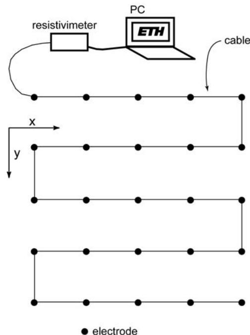
Figure 7: Example of 3D surface electrical tomography (Marescot, 2005-2007)
