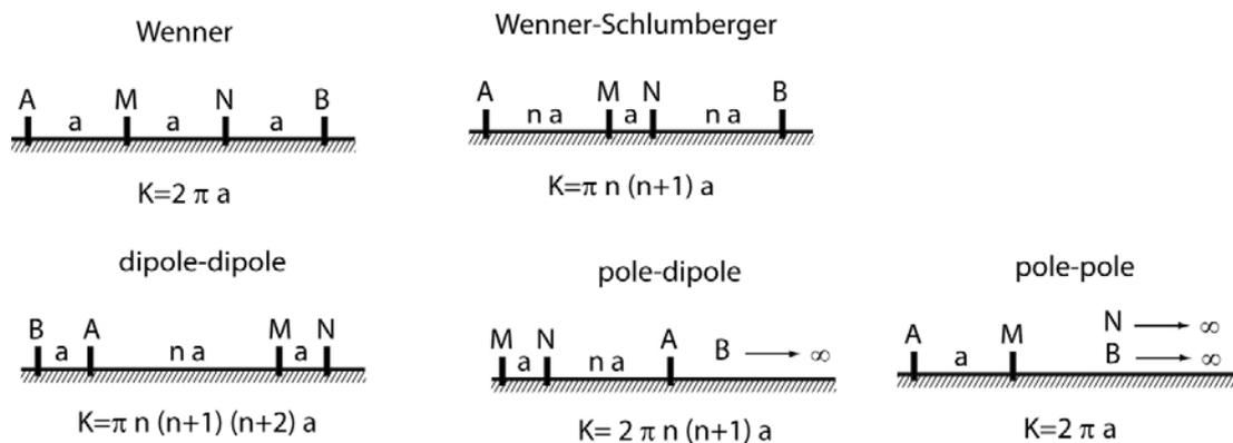
Figure 3: Electrode arrays frequently used in surface electrical prospecting (modified from Marescot, 2006)
