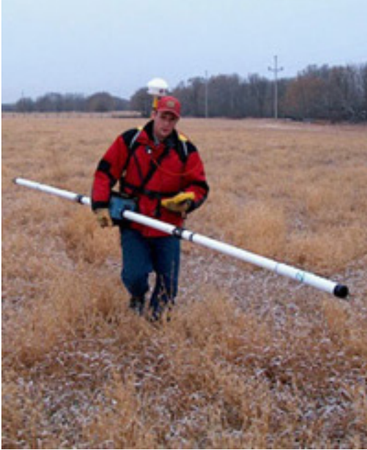
EM31 (Geonics), 9.8 kHz, s=3.66 m
