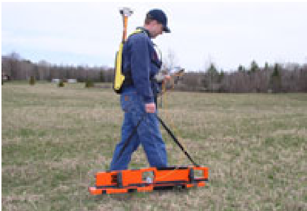
EM38 (Geonics), 14.6 kHz, s=1 m
